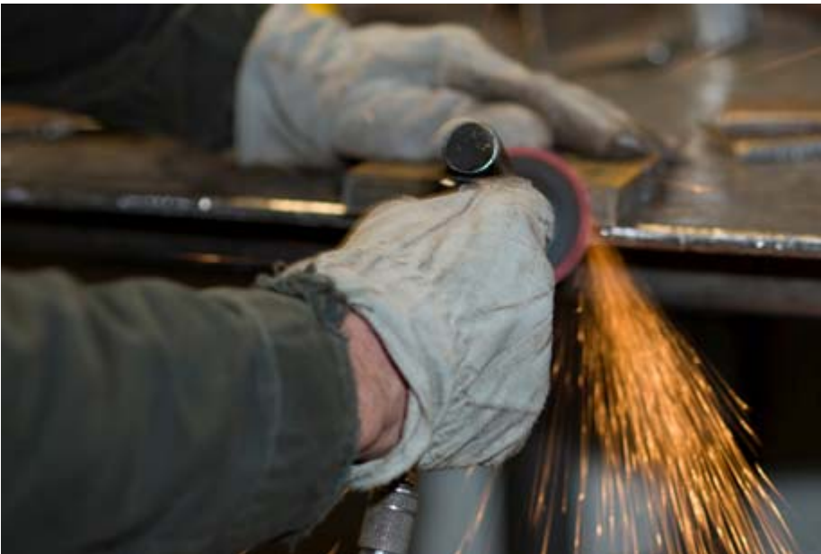
Nathan Szafranski grinds away debris to fabricate a certification plate. A certification test can take up to four hours to complete.
