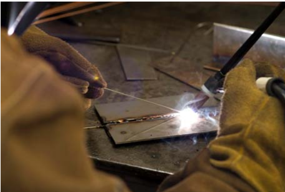
Paul Jones must maintain a specific temperature while he welds stainless steel plates to prevent damage to the metal from heat fluctuations.
