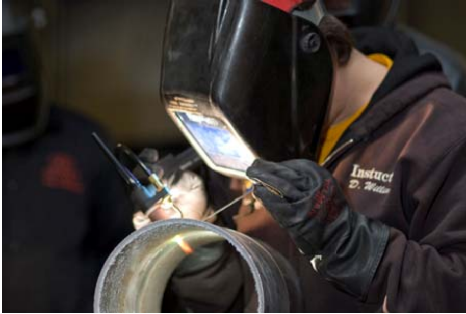
Dave Williams uses tungsten to fuse the aluminum pieces together. Aluminum is a light metal and requires the delicate welding precision of gas tungsten arc welding.
