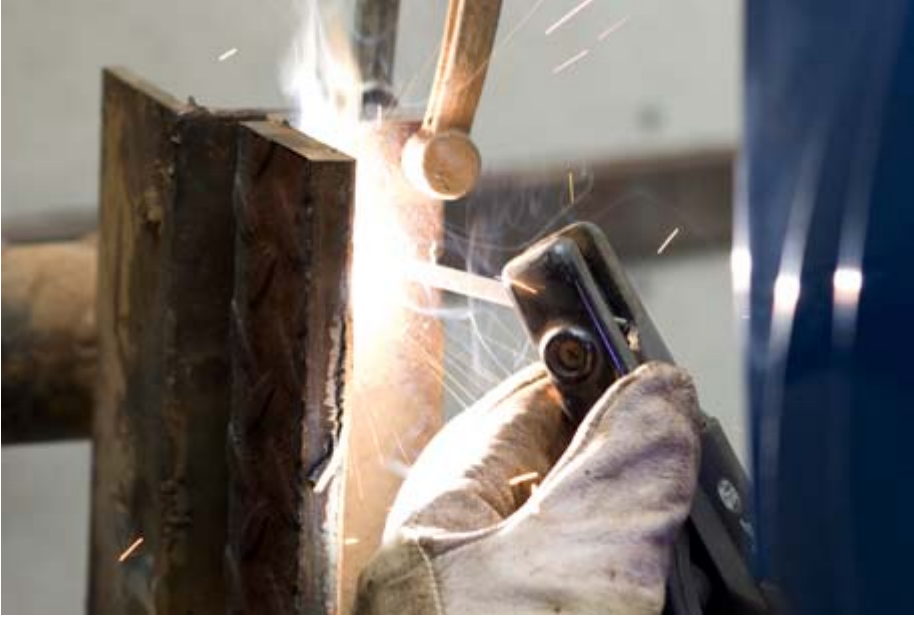
Rupert Reyes must keep the molten metal bead moving upward without dripping to complete a vertical weld.
